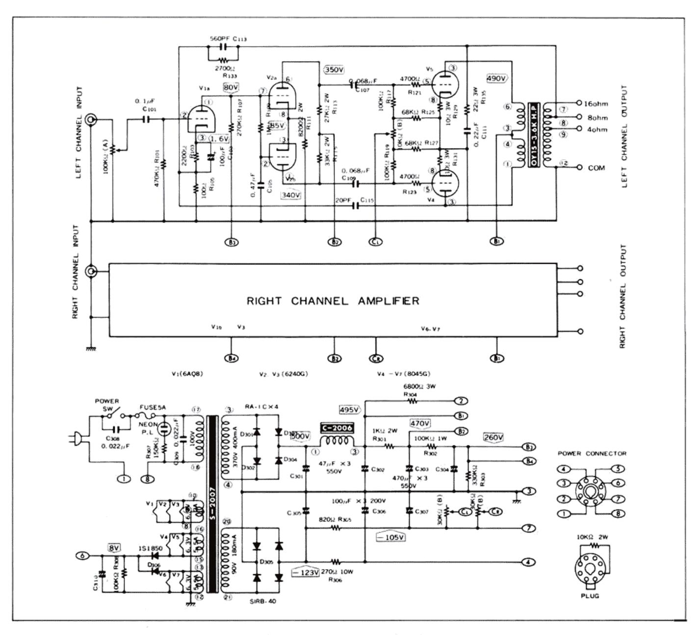
The MQ3600 offers mighty 50 watts RMS output power per channel thanks to class "AB<sub>1</sub>" push-pull operation with the LUX's exclusive giant triode output tube 8045G.
